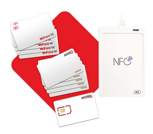
The ACR1552 from ACS is the fourth generation of a very popular NFC Forum-certified, 13.56 MHz USB contactless smartcard reader that supports ISO14443 type A and B cards, MIFARE, FeliCa, and ISO 18092-compliant NFC cards and tags, and now ISO 15693 cards too. Replacing the earlier ACR122 and ACR1252U, this reader is equipped with a SAM slot which provides a high-level of security in contactless and NFC transactions, and can also be supplied in various OEM module formats.
